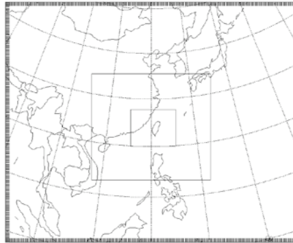
Fig. 3 WRF Inter-nesting model configuration used for Typhoon Moratok case. Horizontal resolutions for domains are 18, 6 and 2 km, respectively.
