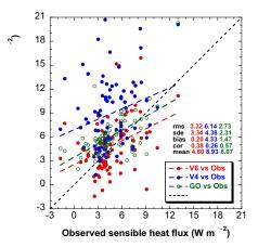
**Figure 5**: The respective Wentz Version 6 (red solid circle) and Version 4 (blue solid triangle) (combined F13 and F14) daily sensible heat flux vs the observed from the five experiments altogether. The daily sensible heat flux ("GO") computed by applying ship data into the GSSTF2 bulk flux model vs the observed is also shown (green open circle).
