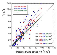
**Figure 6**: The respective Wentz Version 6 (red solid circle) and Version 4 (blue solid triangle) (combined F13 and F14) daily wind stress vs the observed from the five experiments altogether. The daily wind stress ("GO") computed by applying ship data into the GSSTF2 bulk flux model vs the observed is also shown (green open circle).
