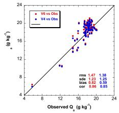
**Figure 3**: The respective Wentz Version 6 (red solid circle) and Version 4 (blue solid triangle) (combined F13 and F14) daily surface air humidity vs the observed from the five experiments altogether.
